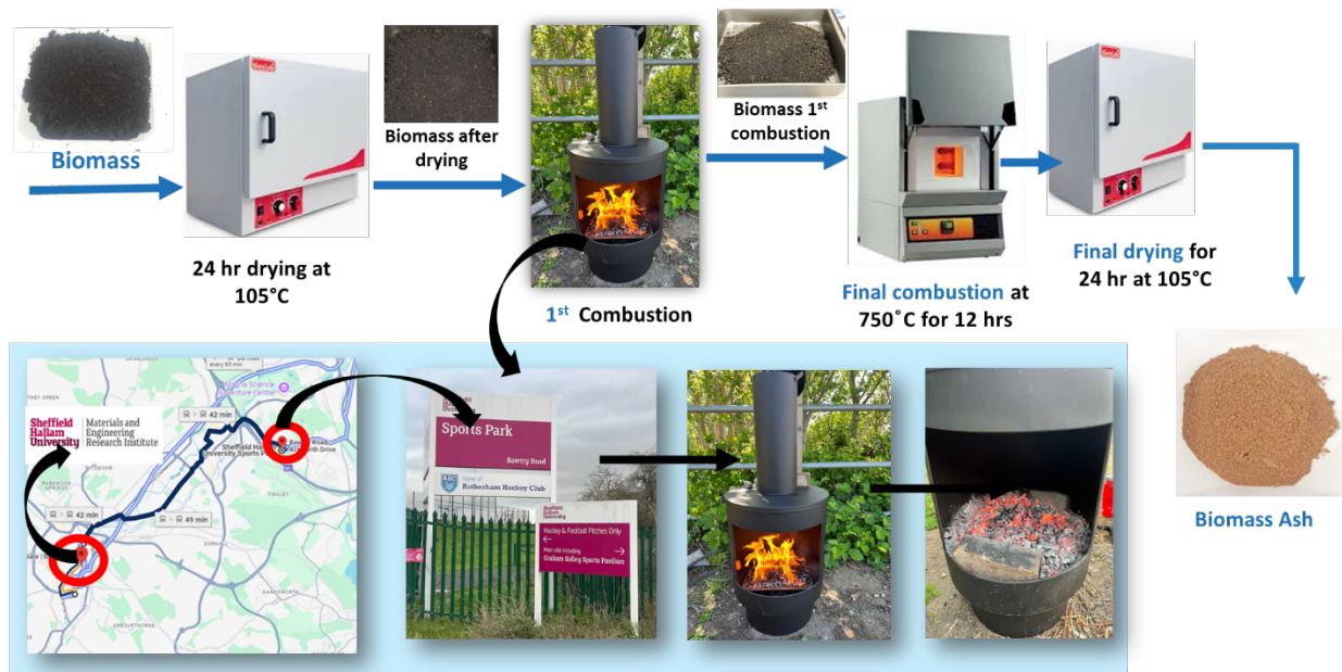
Figure 2.1: Double combustion method to prepare ashes collected from LEI, Lithuanian partners.
